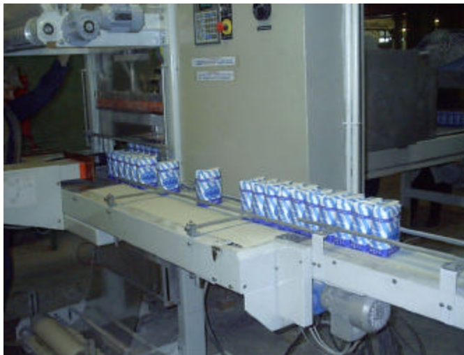
Picture 3. New packaging line for 1 kg paper bags on Mozyrsol
