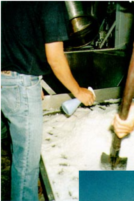
Using a hand-held plant sprayer to iodize salt
