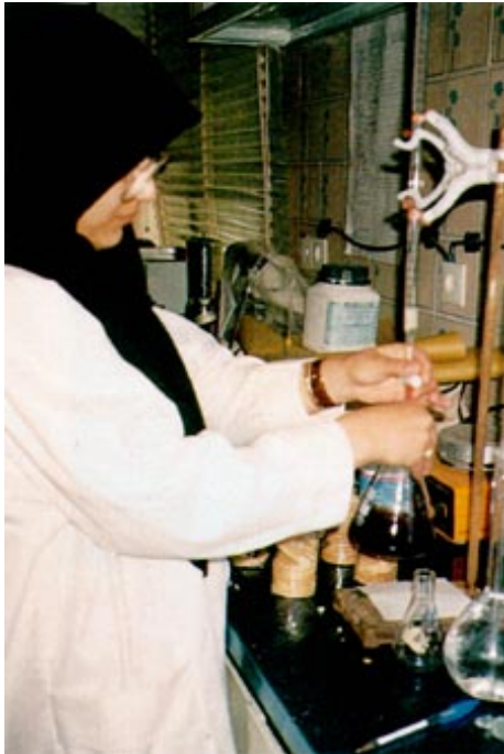
Titrating iodized salt to determine the iodine content
